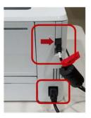
If the ICX-BMD is designated as the accessible voting unit, plug the cable coming from the top left side of the ICX tablet into the top of the ATI then plug the headphones into the "Audio" jack on the bottom of the ATI.
