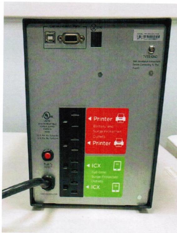
When deployed, a single 15-amp receptacle with no other appliance running on the line can accommodate 3 of the UPS systems. If the receptacle is a 20-amp circuit with no other appliances running, then 4 UPS units can be run on that circuit.
